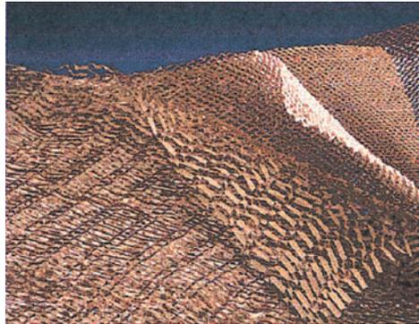
Fig. 1. Expanded paper paint overspray collector.
