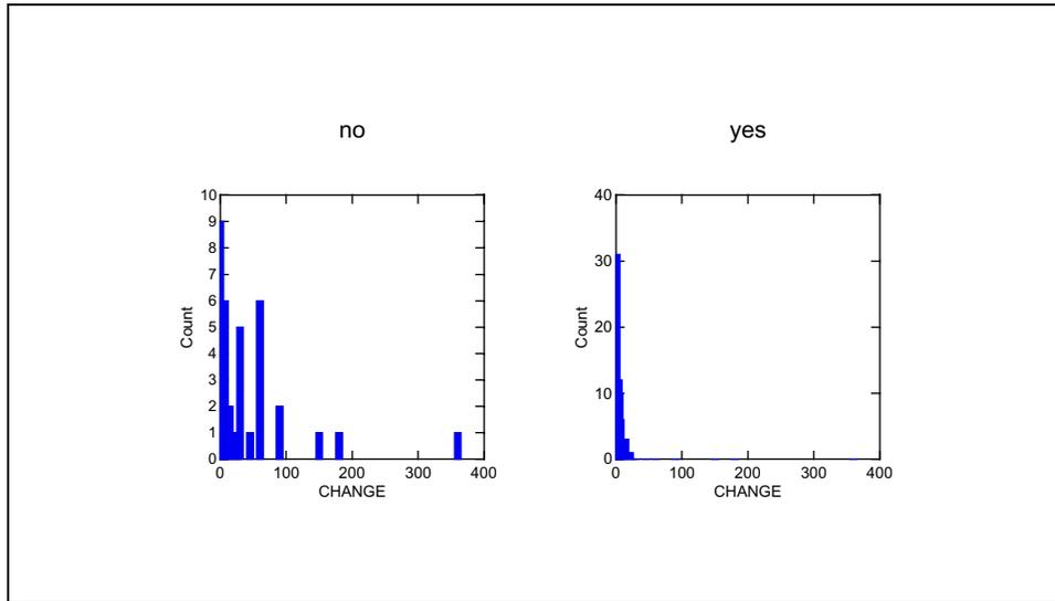
**Figure 5 - Distribution of the interval between filter changes in hours for those facilities that did not experience fires (labeled “no”) and for those facilities that did experience fires (labeled “yes”).**
