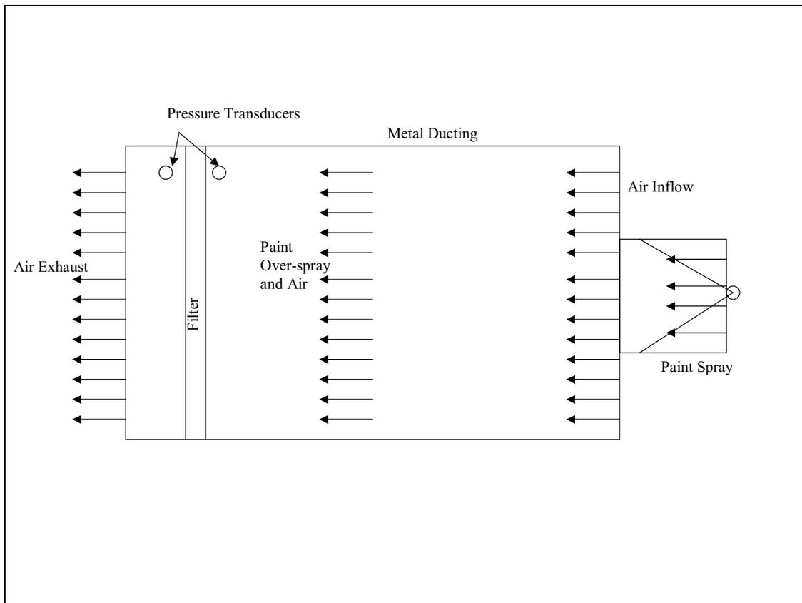
**Figure 7 – General schematic of filter loading apparatus.**
