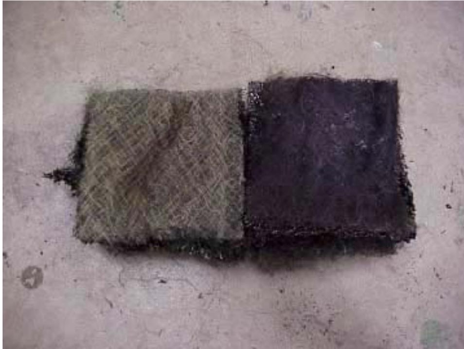
Figure 10 - Paint loaded filter after test (sub-critical).
