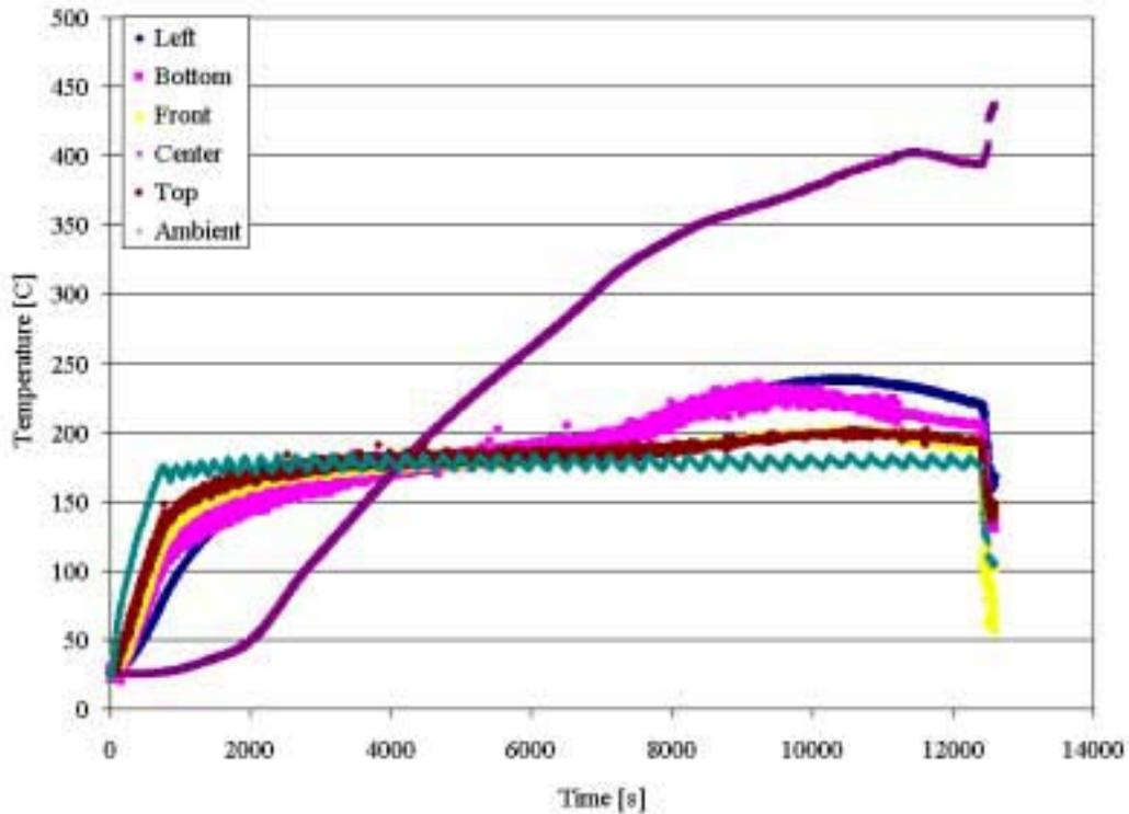
Figure 14 - Ignition of sub-critical sample with added air supply.
