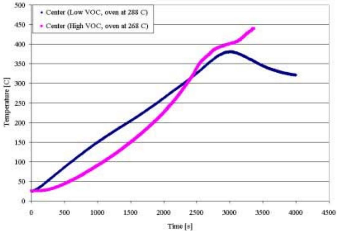
Figure 15 - Significance of VOC content in the paint applied to the filters (4 inch, full load).
